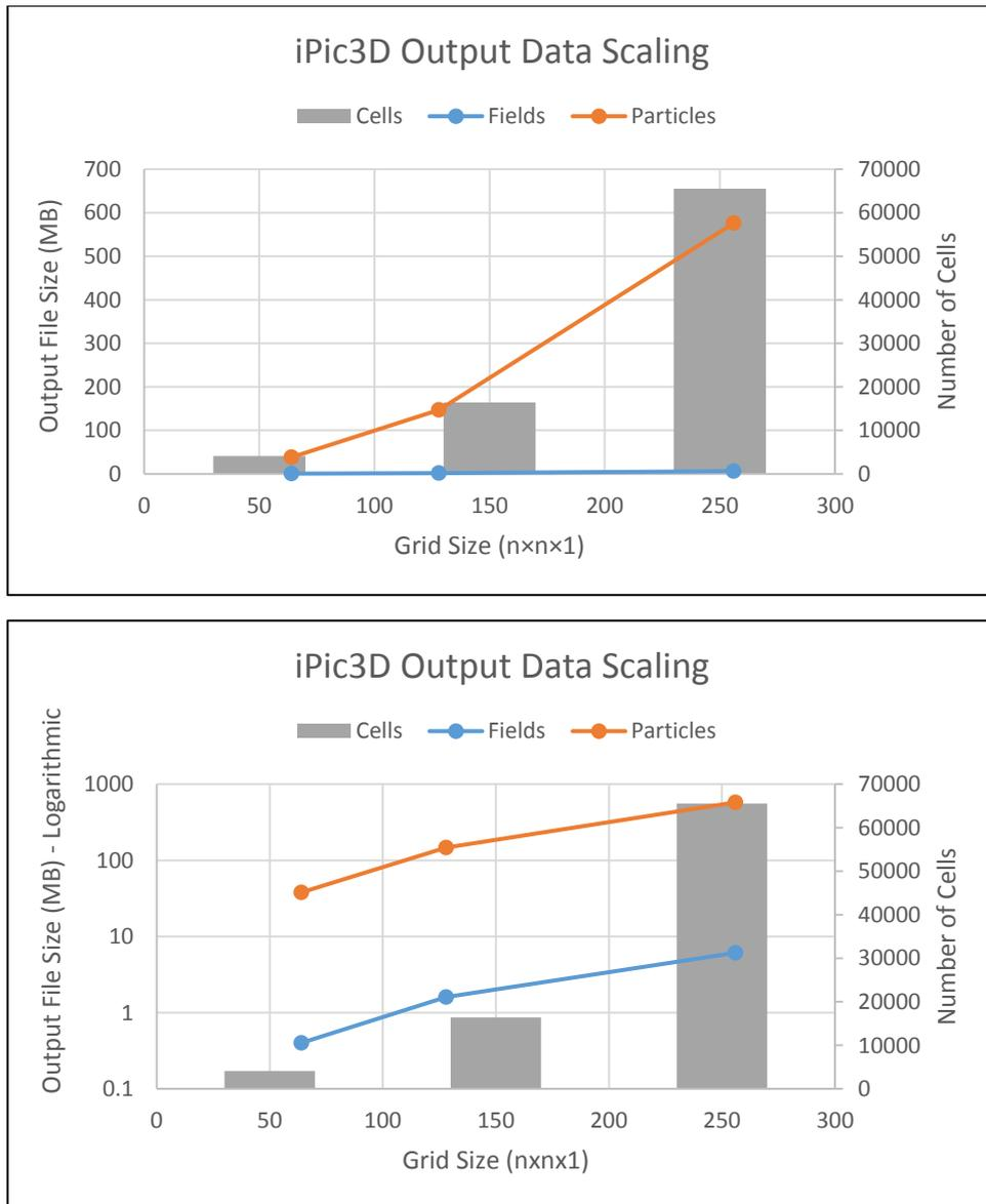
Figure 1: Output file sizes and number of cells as a function of grid size for the iPic3d I/O mock-up. The top chart shows the output file sizes in a linear scale while the bottom chart shows them in a logarithmic scale.
