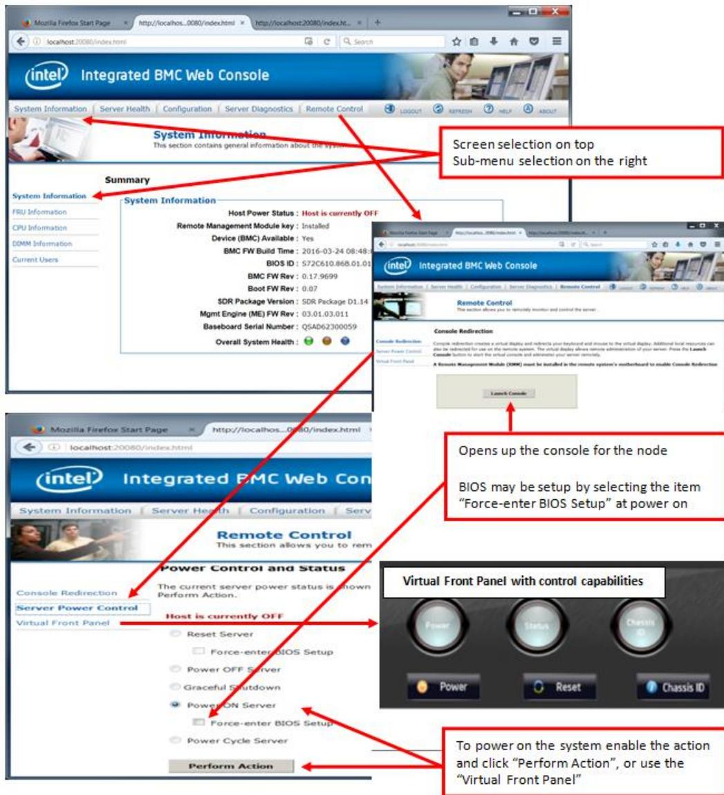
Figure 6. Control procedure using the WEB browser.
